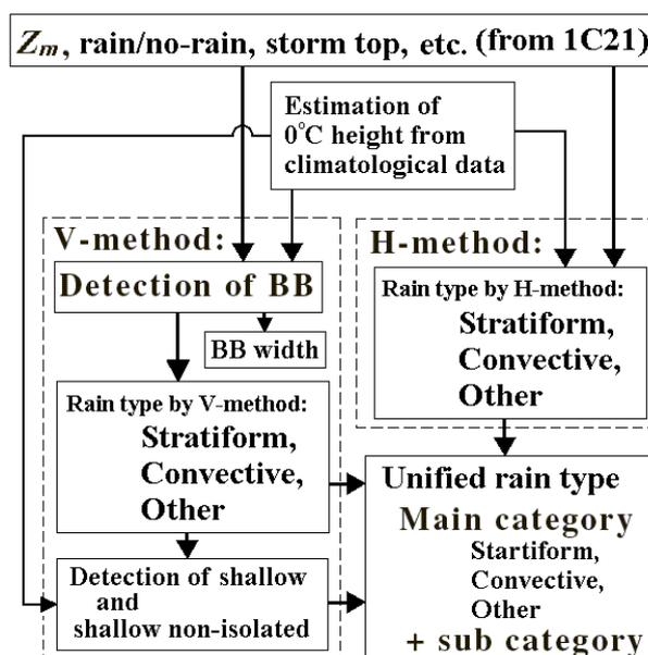
Fig. 1 Flow chart of 2A23 (V6)
